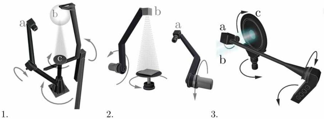
Figure 9. (1) The arrangement of the camera and light source described by Holroyd, et al. (2010). (2) The cumulative adaptive slice measurements described by Filip et al. showing the specular direction *a*. and the anisotropic direction *b* (Filip & Vávra, 2014).
